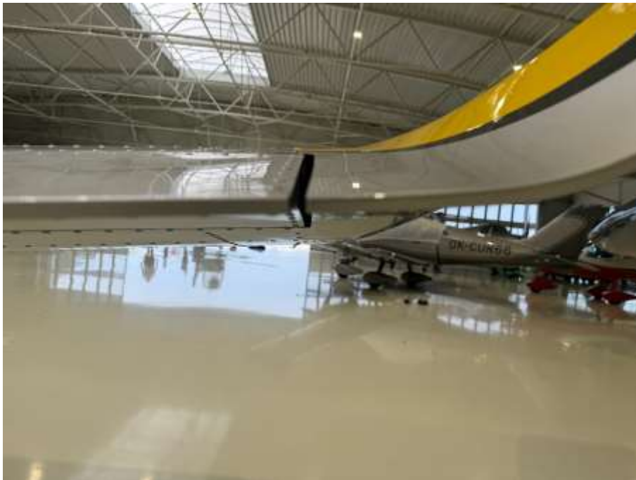
Fig. 6-5 Right aileron trailing edge aligned with the wingtip trailing edge in neutral position. To get this alignment adjust aileron last control rod.
