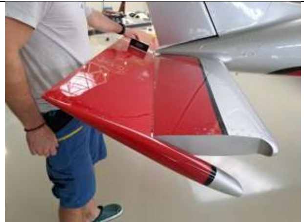
Fig. 6-16 Measure and record elevator up deflection
