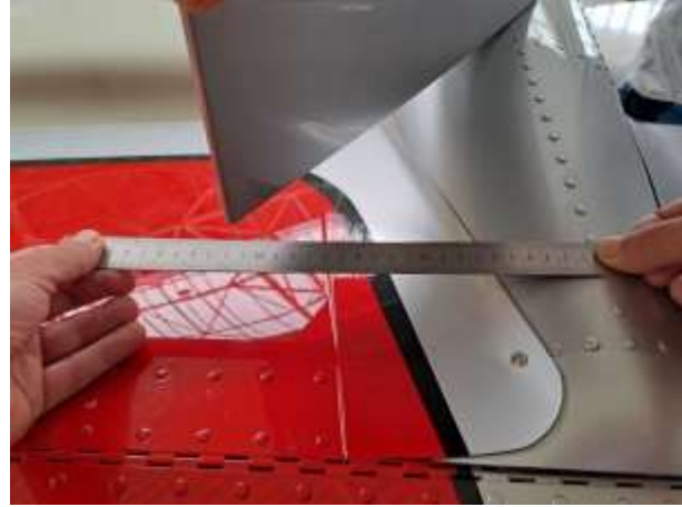
Fig. 6-20 Rudder left deflection. 30° = 225 mm
