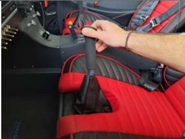
Fig. 6-11 Move the control stick fully right to the stop Repeat the procedure for the right aileron. Measure the deflection at aileron root, not at the tip
