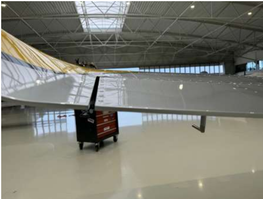
Fig. 6-3 Left aileron trailing edge aligned with the wingtip trailing edge in neutral position. To get this alignment adjust aileron last control rod.
