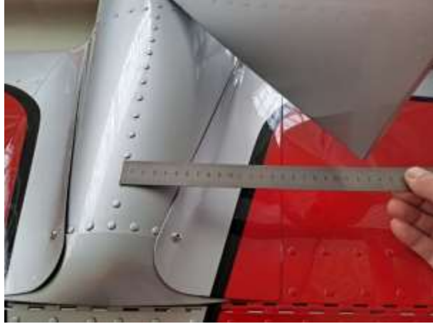
Fig. 6-19 Rudder right deflection. 30° = 225 mm
